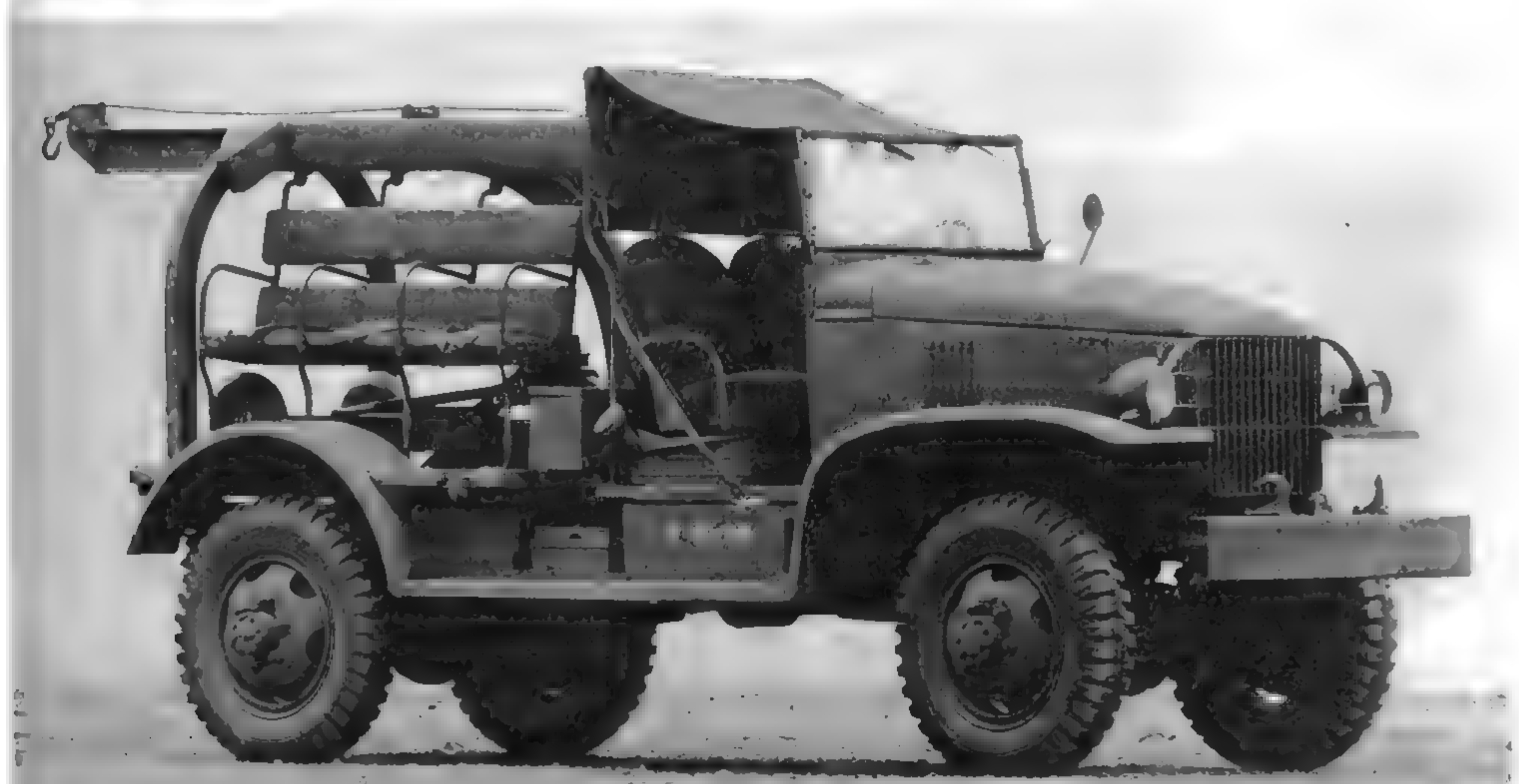
This factory-fresh Bomb Service truck was photographed at the Studebaker Proving Ground in January of 1944. While most of the trucks in the G-506 series were built on 145-in.-wheelbase chassis, these trucks were built on a 125-in. wheelbase, presumably for greater maneuverability in ammo dumps. (U.S. Army photo)
